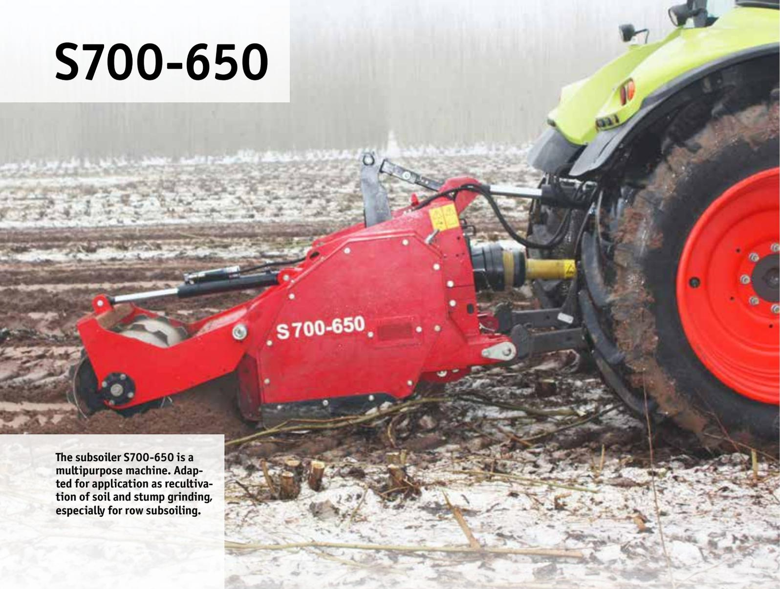
The subsoiler S700-650 is a multipurpose machine. Adapted for application as recultivation of soil and stump grinding, especially for row subsoiling.
