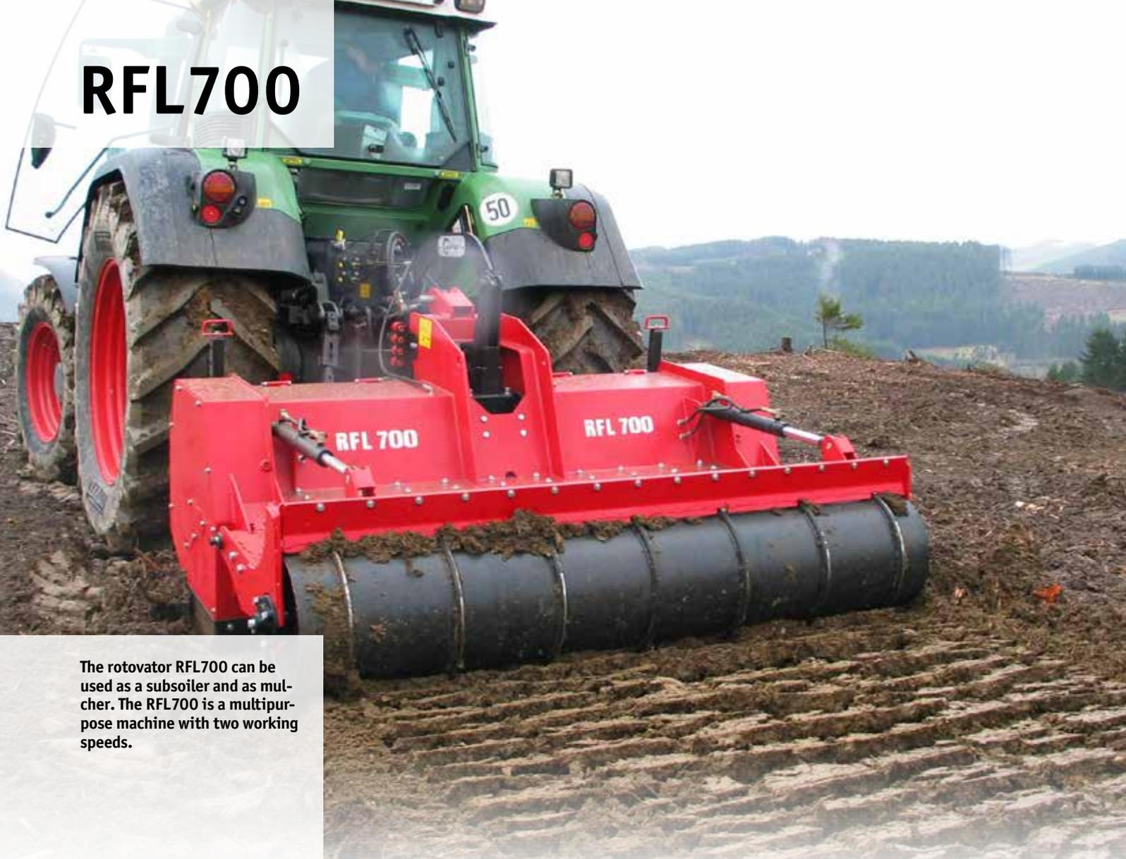
The rotovator RFL700 can be used as a subsoiler and as mulcher. The RFL700 is a multipurpose machine with two working speeds.
